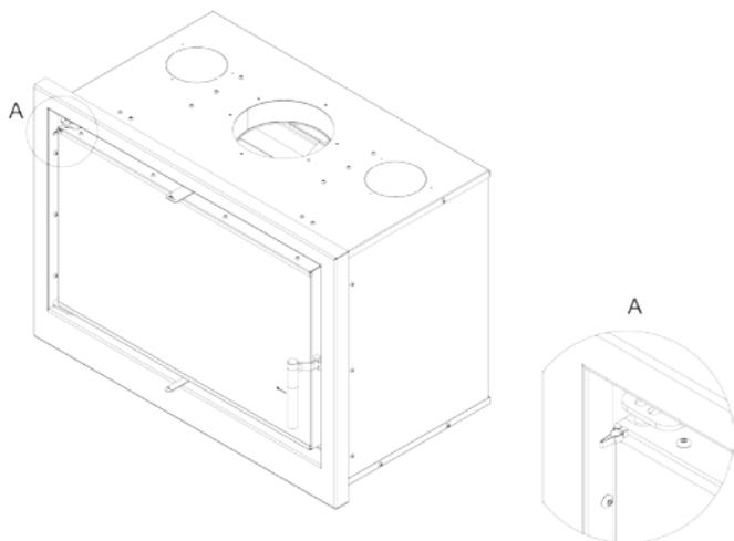
Fig. 7. RK cassette - dismantling the door, step 1
