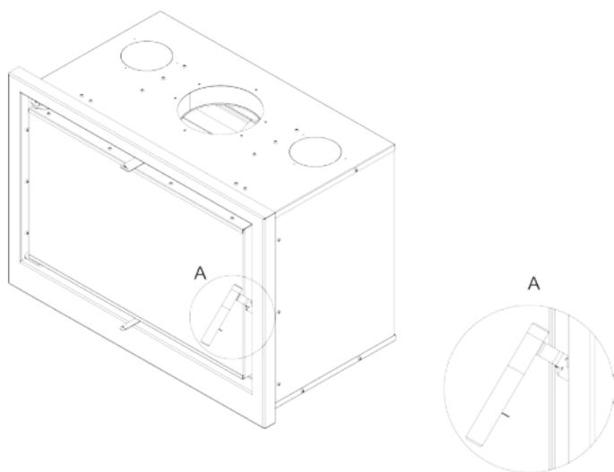
Fig. 8. RK cassette - dismantling the door, step 2
