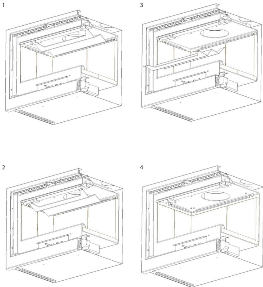
Fig. 13. RK cassette - dismantling the deflector and the slats holding the Acumote
